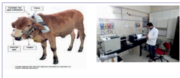
Analysis of methane and SF 6 gas using Gas chromatography
