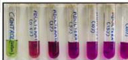
Indicator 1 with increasing concentration of sorbitol in water + 0.5% boric acid n=8
